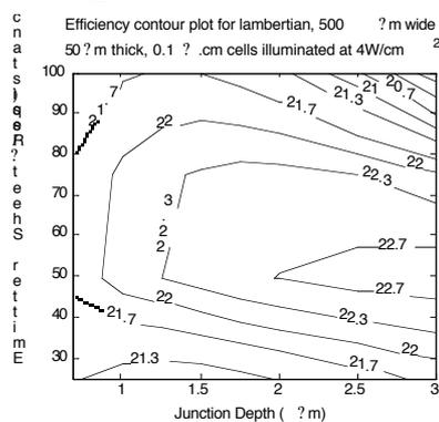
**Figure 7:** Effect of emitter diffusion magnitude and depth (for Gaussian profile) on cell efficiency.
