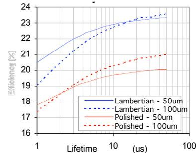
Figure 6: Efficiency versus carrier lifetime for cells with 0.1  $\Omega$  .cm bulk resistivity.
