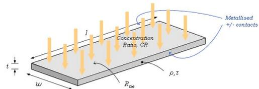
**Figure 2:** Concentrator Sliver® cell with modelled design parameters shown.
