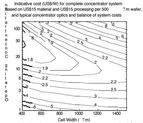
Figure 11: Projected total system costs (US\$/W) for concentrator Sliver® cell system, based on cost model.
