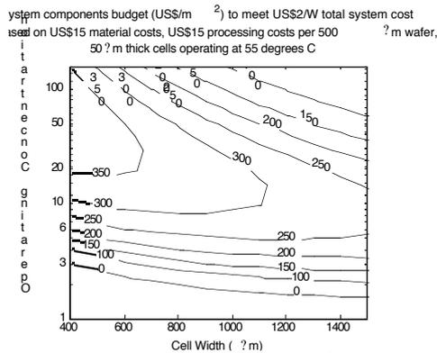
Figure 9: System components budget for US\$2/W total system cost.
