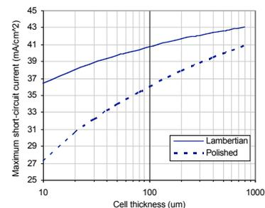
**Figure 3 .** Maximum Sliver® cell short circuit current for light trapping scenarios with lambertian and polished surfaces.
