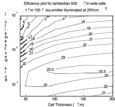
Figure 5: Efficiency for a range of bulk resistivity and cell thicknesses.
