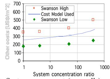
Figure 10: System component (non-cells) cost model.
