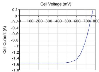
Figure 3. IV curve of a modelled cell at 4W/cm<sup>2</sup>
