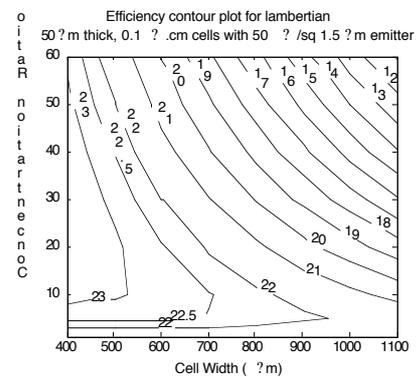
**Figure 8:** Dependence of cell efficiency on cell width and concentration ratio
